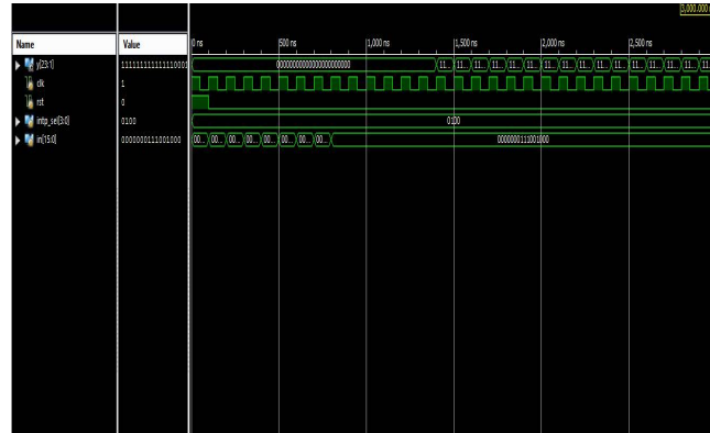
Fig 9 : Waveform of Decimation Filter
