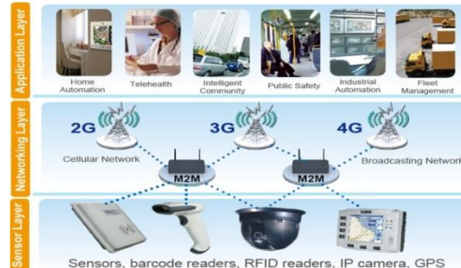
Figure 3.IOT architecture with example devices in each layer [10]
