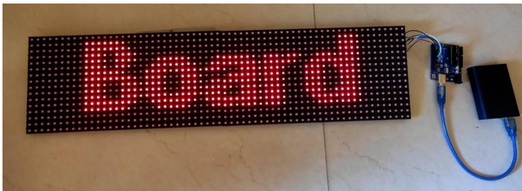
Fig. Message displayed on P10 LED matrix display
