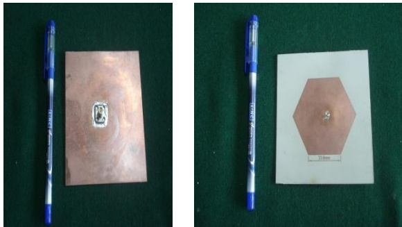
Fig.20 Fabricated Antenna a) Ground Plane(left), bottom view b) Hexagonal Patch, Top View(Right)
