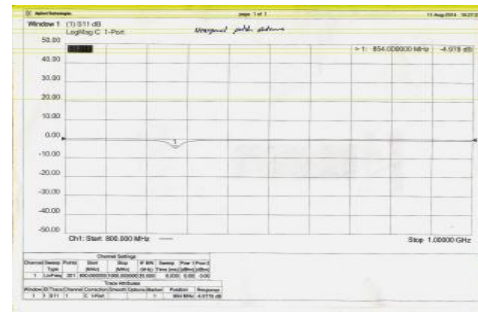
Fig.21 Return Loss S_{11} (dB) Vs Frequency (MHz) (Left) (b) Measured in Network Analyzer (Right)
