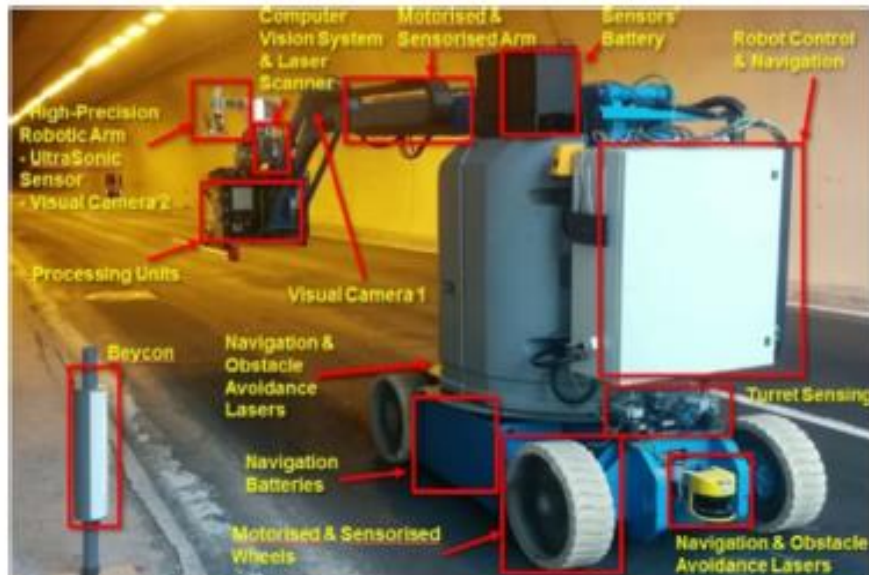
Figure 1: The components of the robo-spect robotic platform
