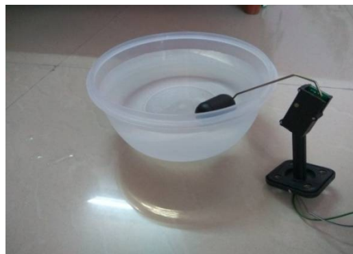
Fig 6: Level Sensor Plotted in a Bowl
