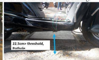
Fig 8c. Detection of pothole.
