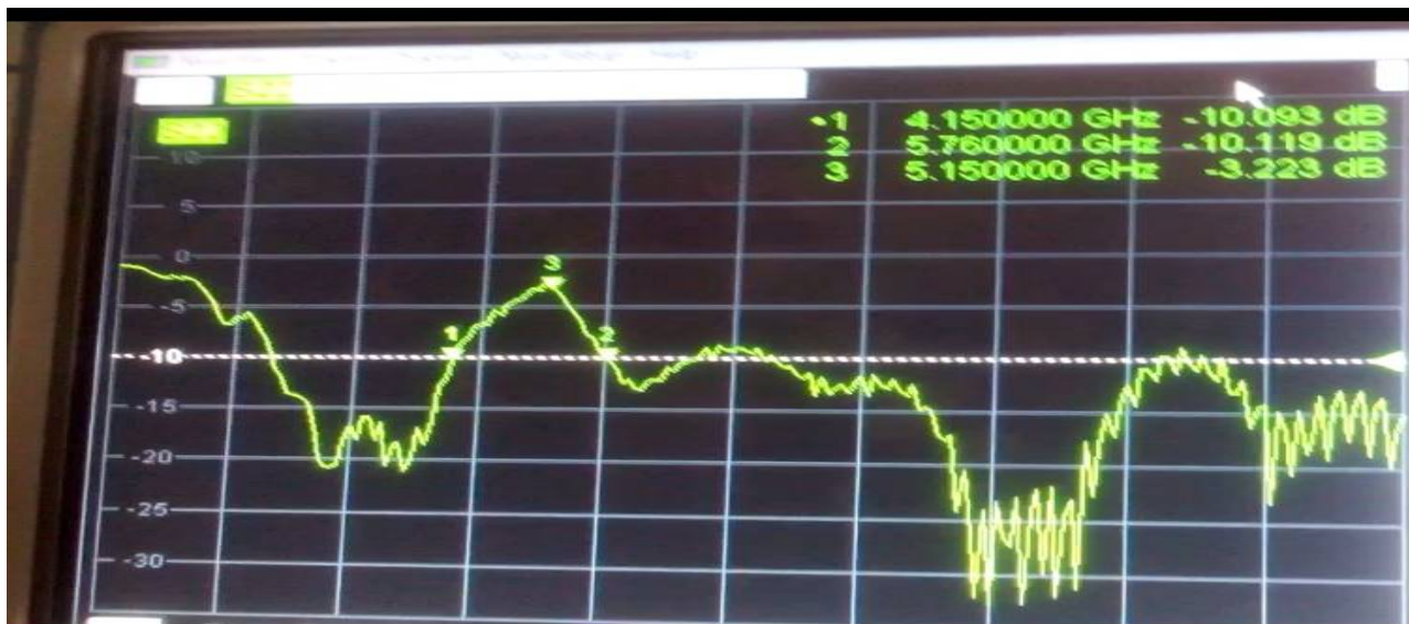
Fig.10. Return loss Measured on Network Analyzer
