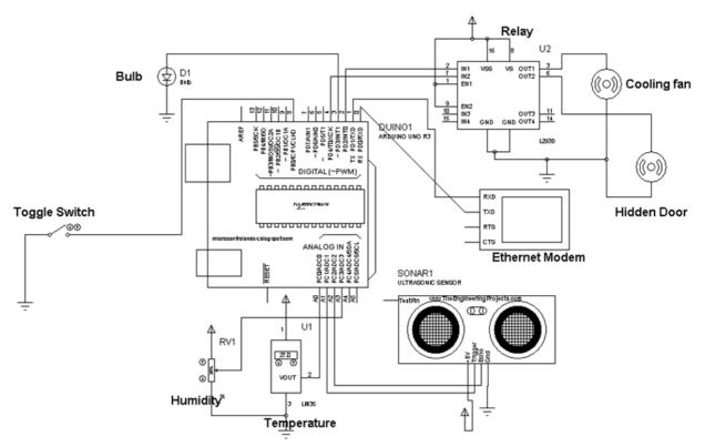
The Arduino Uno is a microcontroller board in light of the ATmega328. It has 14 computerized input/yield pins (of which 6 can be utilized as PWM yields), 6 simple information sources, a 16 MHz precious stone oscillator, a USB association, a power jack, an ICSP header, and a reset catch. Arduino contains everything expected to bolster the microcontroller; just interfaced to a PC with a USB link or power it with an AC-to-DC connector or battery to begin.
