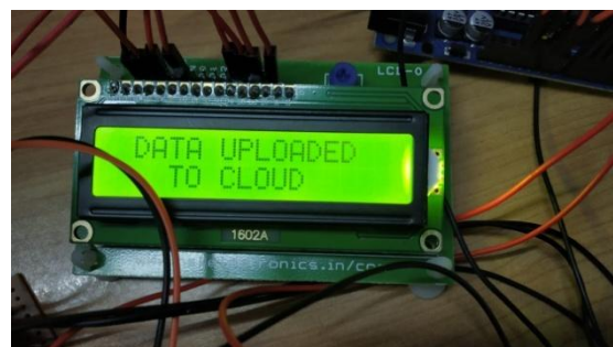
Fig 4.4: Uploading voltage and battery status to the cloud
