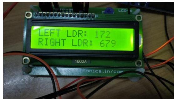
Fig 4.2: Tracking of solar rays on the LDR sensors
