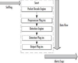
processors function is to take packets potentially dangerous for the detection engine to try to find known patterns. Preprocessors can alert on, classify, or drop a packet before sending it to detection engine
