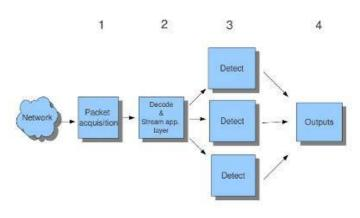
Suricata consists of a few modules like Capturing, Collection, Decoding, Detection and Output. It captures traffic passing in one flow before decoding, which is highly optimal. It configures separate flows after capturing and specifying how the flow will separate between processors.
