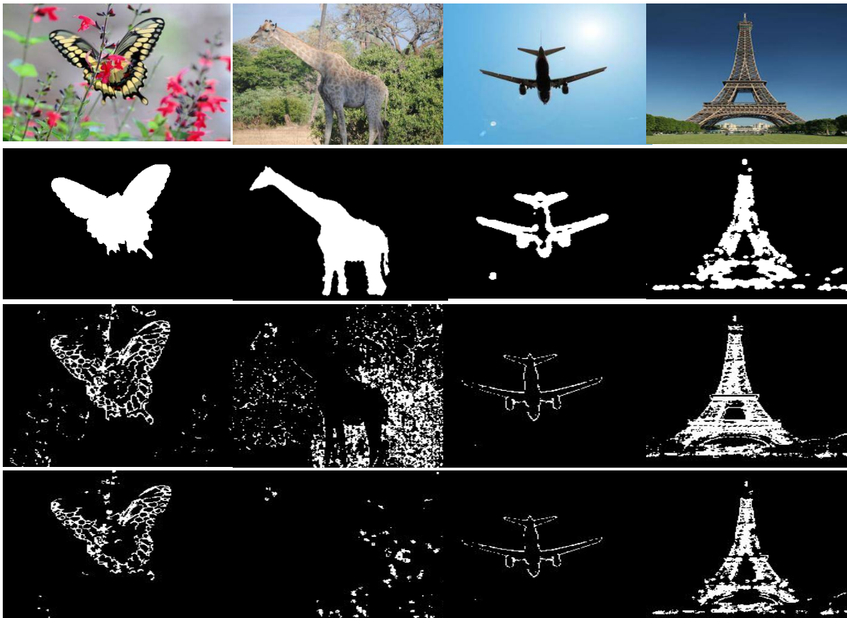
Fig 2: Example of contour maps. First row is the natural image. Second row is the salient region of the images. Third row is global contour maps and the forth row is salient contour maps.
