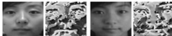
Fig 1: Examples of two images (a live face and a face print) in the original space and the corresponding LBP images using LBP as a feature space [7].
