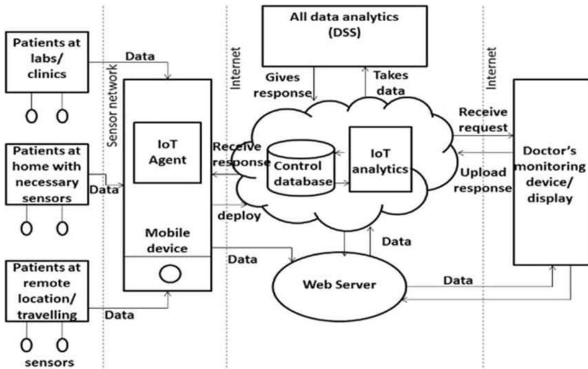
(fig1).Architecture of Healthcare Monitoring System
