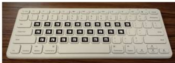
Fig. 3. A QWERTY keyboard with alphabetic markers glued on top of the corresponding alphabet keys.
