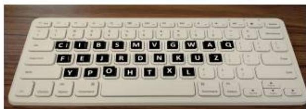
Fig. 4. An instance of an augmented keyboard with IKR strategy as observed by the typer on the EPSON Moverio BT-200.
