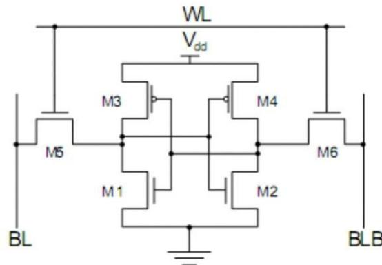
The most commonly used memory cell structure in digital designs is the 6T Conventional SRAM cell. It is called "6T" because it consists of six transistors that store one bit of data. A general model of a 6T SRAM can be viewed as a latch made up of two cross-coupled inverters and two access transistors, which control the read and write operations[2].
