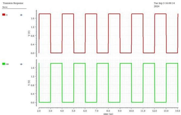
Figure 3- simulation result for 10T SRAM cell.
