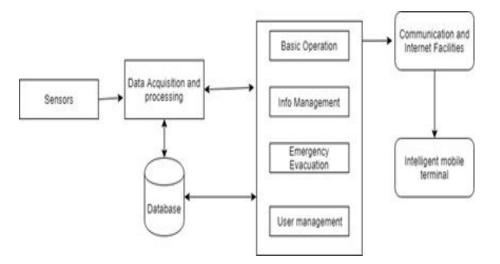
The block diagram of the system, where the current position of the evacuee will be tracked using indoor positioning with the help of a WIFI signal and leads to the short and safe exit.
