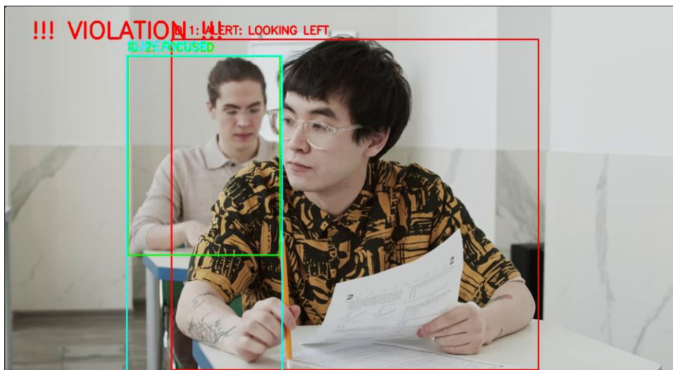
Fig.1. Violation detection: System flagging "Looking Left" based on Yaw angle deviation.
