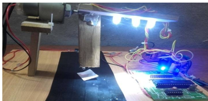
fig(10):Low intensity light when pot is in maximum position
