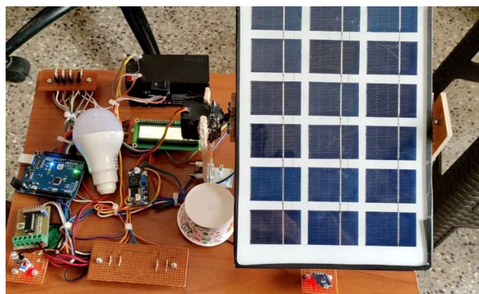
Fig. 3 Initial Stage of smart Street Light System
