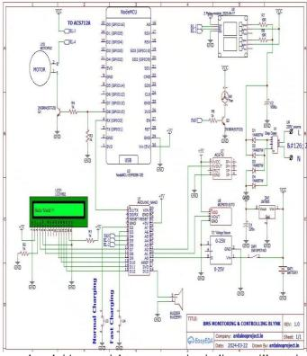
Once all the components are gathered, it's essential to create a circuit diagram illustrating how each component is connected to the ESP32 microcontroller. The circuit diagram serves as a visual guide for the assembly process and ensures proper wiring and connectivity.
