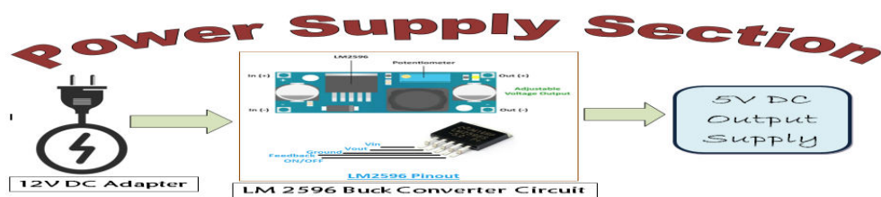
FIG1: power supply section
