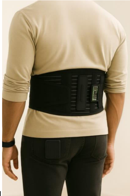
Fig. 4. User wearing the lumbosacral corset. The belt fits on the lower back with the embedded sensing and monitoring system.
