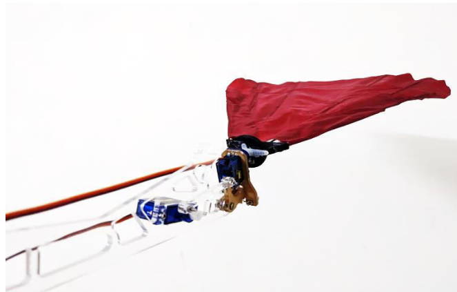
Tail design which is mainly responsible for control of flight
