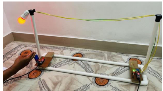
Fig.7 Turning off the overhead lines using RF Card
