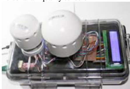
The Air Quality Egg: An example of a low-cost, personal air pollution sensor
