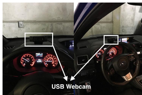
Mounting camera to car dash for drowsiness detection
