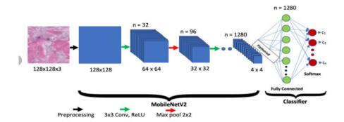
The network consists of 28 convolutional layers and 1 fully connected layer followed by a softmax layer.
