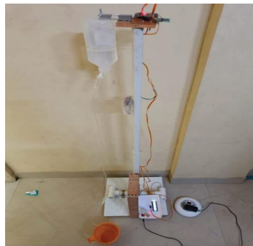
Fig: IV Pole Monitoring Prototype
