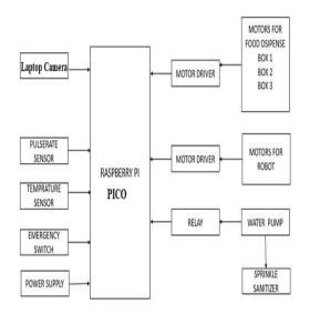
The Parental Caring Robot operates as an intelligent system designed to monitor, interact with, and assist children. The system integrates various hardware components and intelligent features, managed by a Raspberry Pi Pico, to provide a seamless care giving experience. The working of the robot can be broken down into the following components and functionalities:
