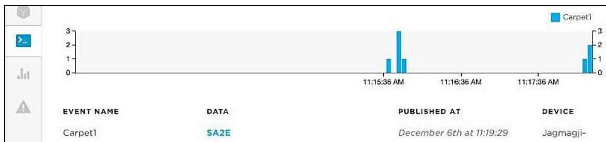
Fig 2(a). The cloud Dashboard displaying the event name Carpet1, sensor data for the lab entrance (sensor 2 was activated), a timestamp, and the device name.
