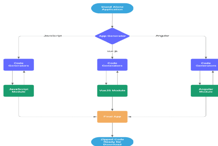
Fig:2 The Schematic block diagram of the App Gen as. standalone application
