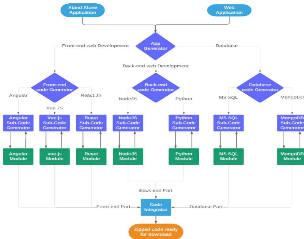
Fig:1 The Schematic block diagram of the App Gen
