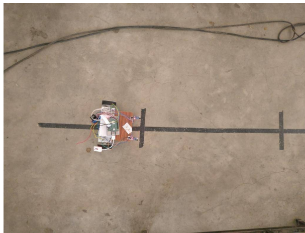
Initialising black line following robot
