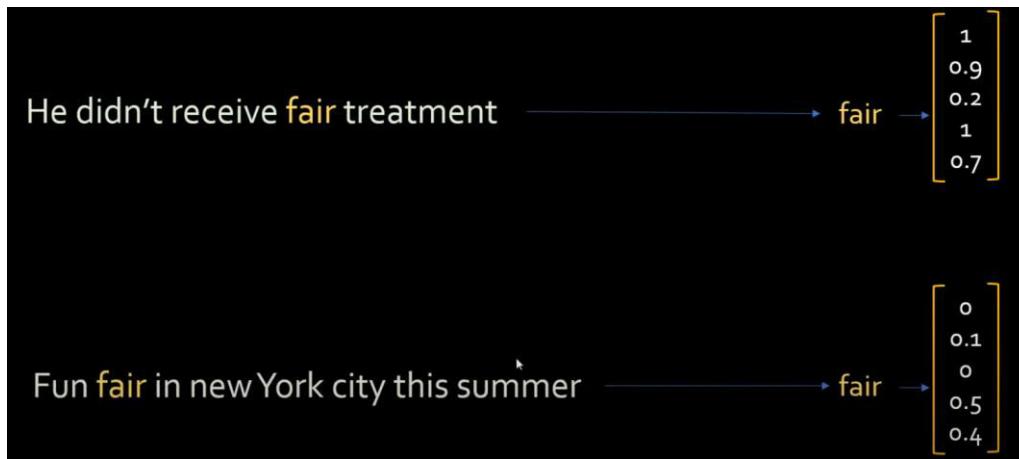
Fig. 2 Context-based models produce different word embeddings for the word ‘fair’ on the basis of their context in the sentences
