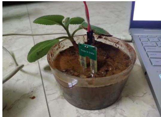
Fig.A.9 Soil moisture is measured through the Sensor
