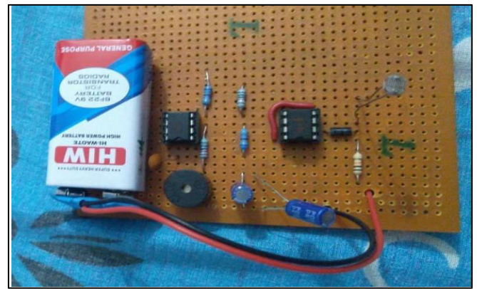
Figure 2: Circuit Implementation on zero PCB.
