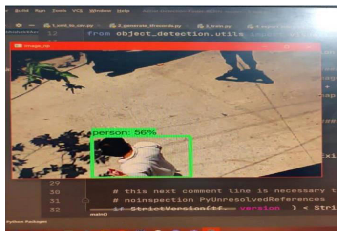
Fig.2(a): Human detection using images captured by drone along with probability/efficiency of detection
