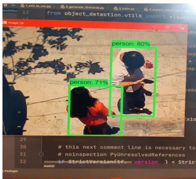
Fig.2(a): Human detection using images captured by drone along with probability/efficiency of detection
