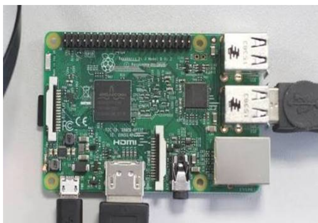
Fig.2 Raspberry pi model B board
