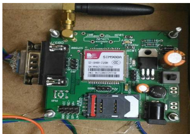
Fig.3 GSM modem board
