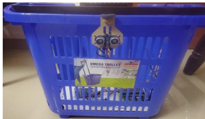
Fig .5 Ultrasonic sensor fitted in Trolley
