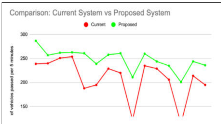
Figure 4: Simulation result analysis of Current System Vs Proposed System
