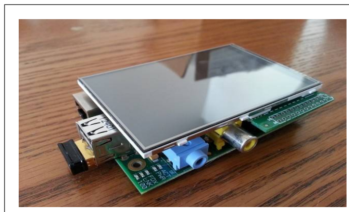
Fig.3: Connection between LCD and Raspberry Pi
