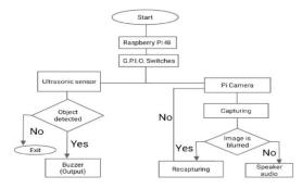
The reading proficiency device is used for conversion of text image to speech and for the object detection using ultrasonic sensor. Basically, this device works in two modes –
