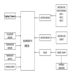
The Parental Caring Robot operates as an intelligent system designed to monitor, interact with, and assist children. The system integrates various hardware components and intelligent features, managed by a Raspberry Pi Pico, to provide a seamless care giving experience. The working of the robot can be broken down into the following components and functionalities:
