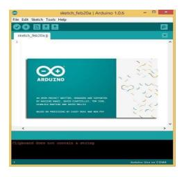
The Arduino Integrated Development Environment (IDE), sometimes known as the Arduino Software (IDE), has a code editor, a message area, a text console, a toolbar with buttons for basic functions, and a series of menus. It communicates with and uploads programmes to the Arduino hardware.
