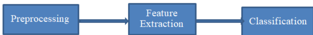
Figure 1: Basic Model of a Speaker Recognition System
