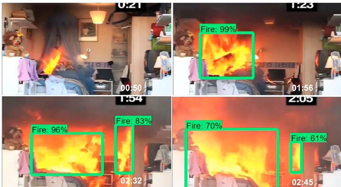
Fig. 1 Fire Is Detected
