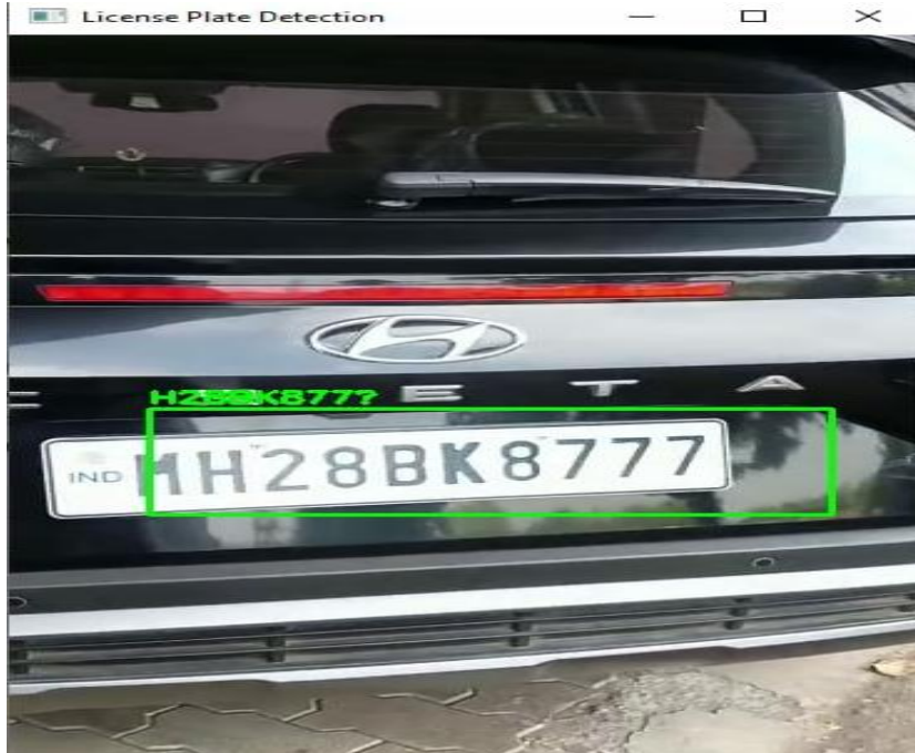
Figure 4: Number Plate Detection using OpenCV
