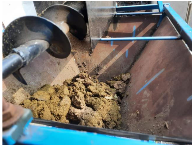
Figure 4: Hopper for feeding cow dung.
