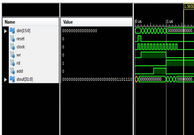
Fig. 8: Simulation Result of 4-tap micro-programmed sequential FIR filter using 16- bit Vedic multiplier
