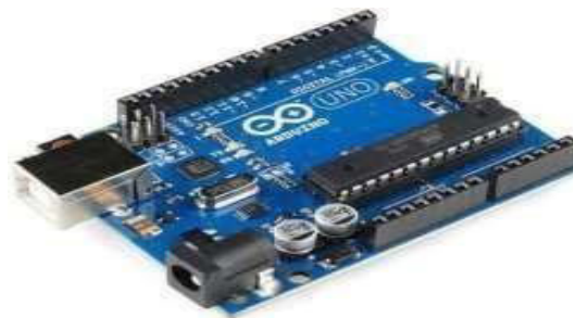
Fig. 2: Arduino board having ATmega 328P Microcontroller.
